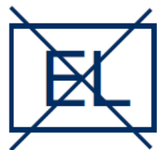
Lamp not suitable for emergency operation
