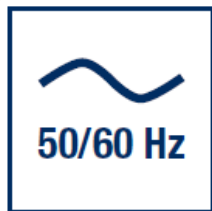
Lamp suitable for 50 Hz or 60 Hz operation
