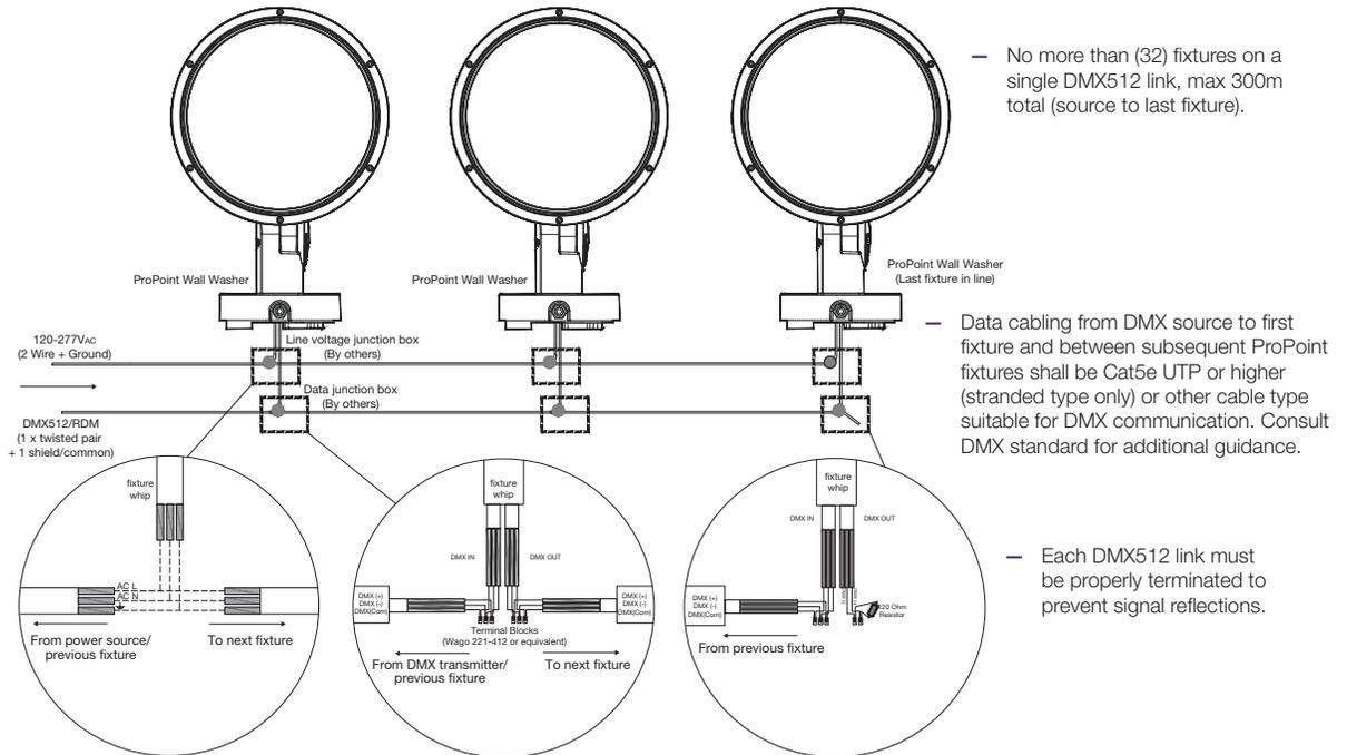
— No more than (32) fixtures on a single DMX512 link, max 300m total (source to last fixture).
